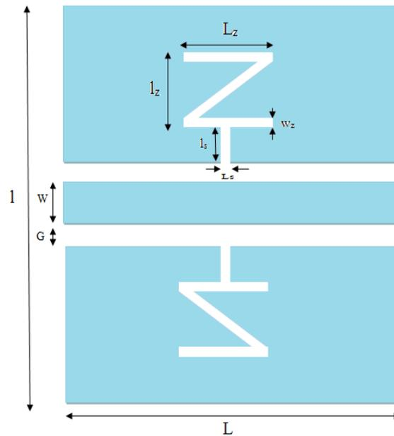
Figure 4. Structure of CPW stopband filter with Z-DGS
