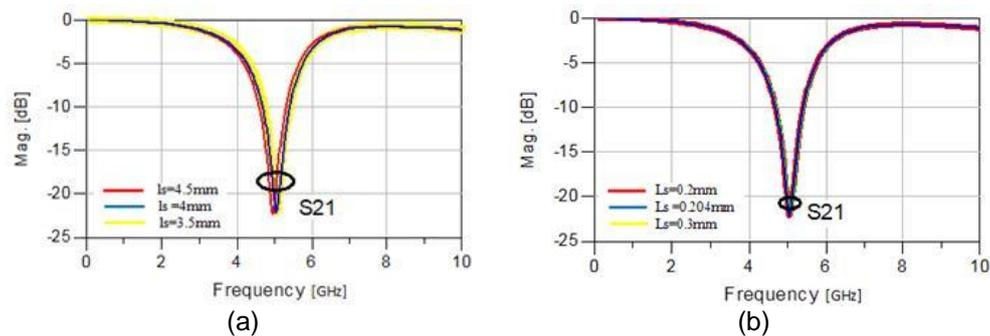
Figure 6. S-parameters of Z-DGS stopband filter: (a) Effect of variation of the length  $l_s$ , (b) Effect of variation of the width  $L_s$
