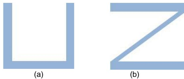
Figure 1. Different DGS geometries: (a) u-shaped DGS, (b) the proposed Z-DGS
