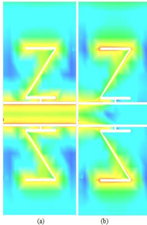
Figure 9. Simulated surface current density: (a) At  $f=2\text{GHz}$ , (b) At  $f=5\text{GHz}$
