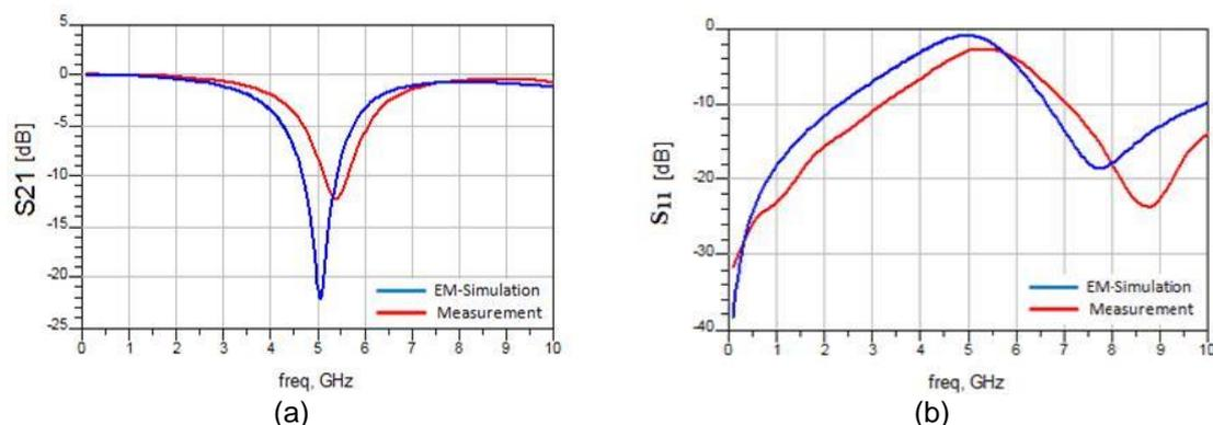
Figure 11. Comparison between the measured and simulated results.
