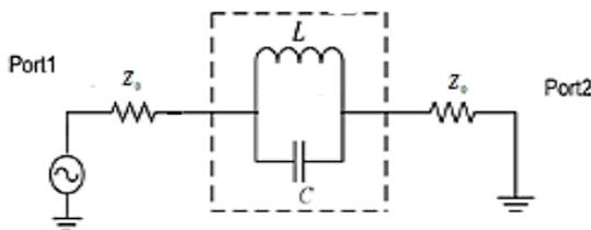
Figure 2. LC-equivalent circuit for Z-DGS resonator
