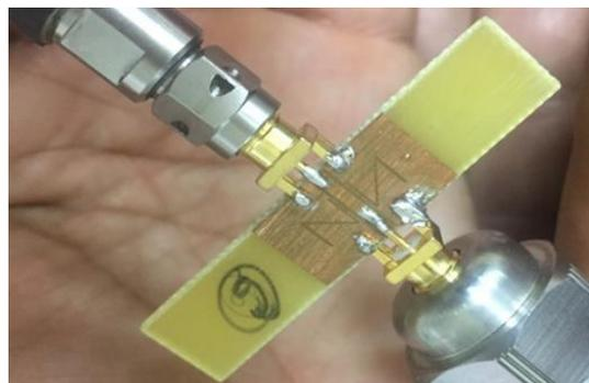
Figure 10. The photograph of the proposed Z-DGS bandstop filter
