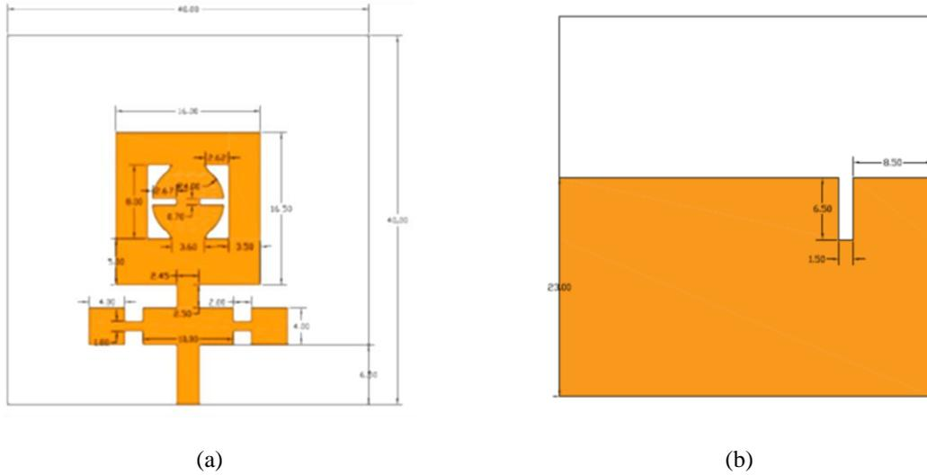
Figure 2. Geometry of the proposed filtering antenna with its optimized dimensions: (a) top view, (b) bottom view
