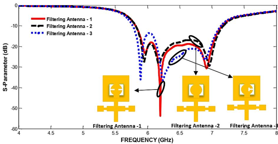
Figure 6.  $S_{11}$ -parameter of the proposed filtering antenna for different shaped slots
