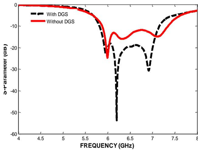
Figure 5.  $S_{11}$ -parameter of the proposed filtering antenna with and without DGS
