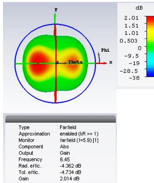
Figure 7. 3-D view radiation pattern of the proposed filtering antenna at  $f_o = 6.45$  GHz
