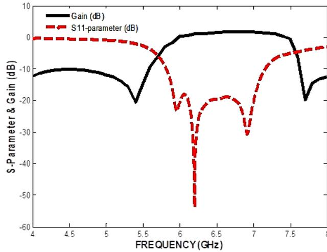
Figure 4.  $S_{11}$ -parameter and gain of the proposed filtering antenna
