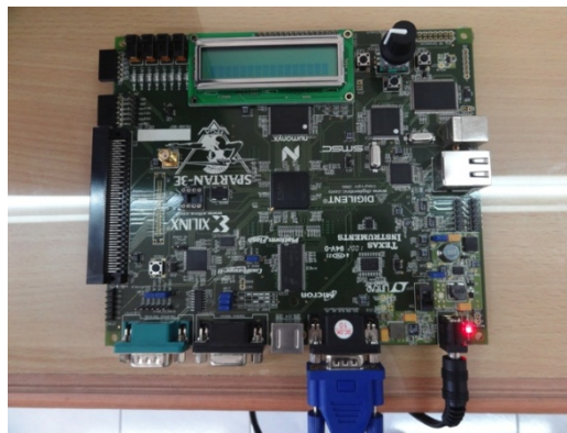
Figure 4. Xilinx Spartan 3E FPGA module is connected to monitor
