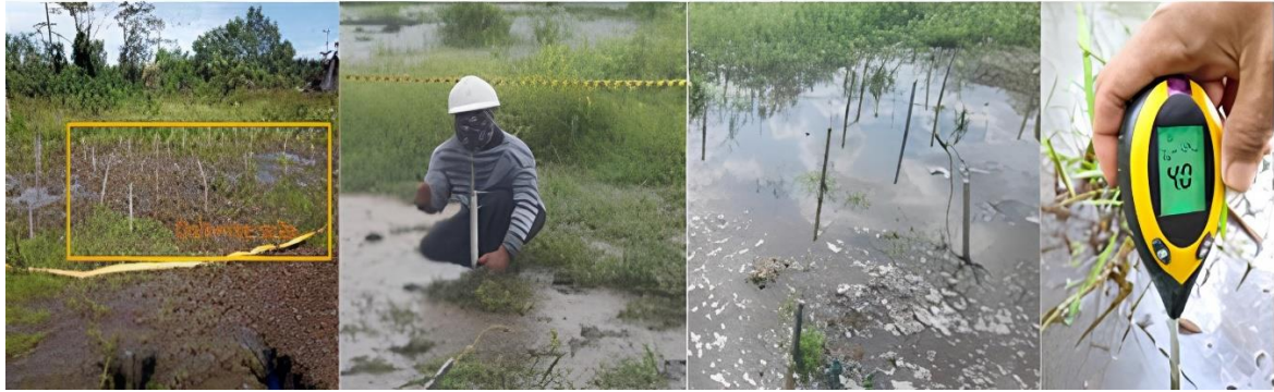
Figure 2. Grounding resistance reduction study with dolomite in acidic water swamp
