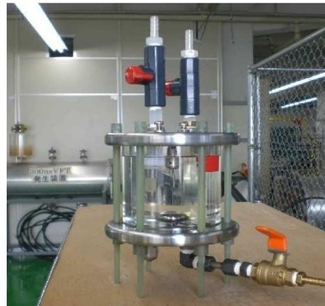
Two terminals at the top of chamber were used to enter the oil sample into the chamber and for vacuuming process, and the other one at the bottom of chamber was used to dispose the oil after measurement.
