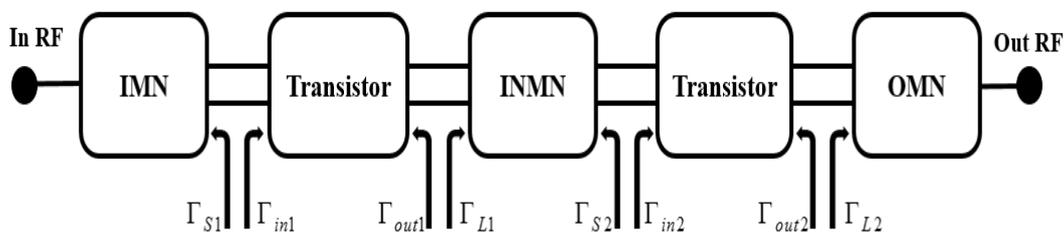
Figure 1. Block diagram of two stages power amplifier
