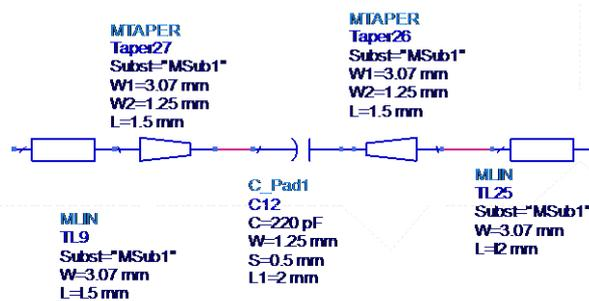
Figure 2(c). Inter-stage matching network circuit
