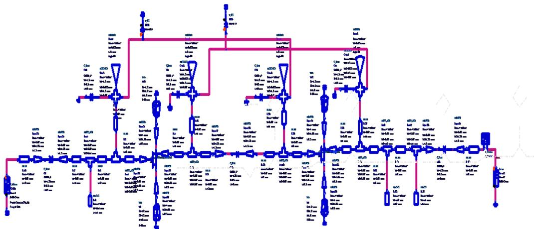
Figure 2. Schematic of the proposed two stage PA circuit using microstrip lines technology
