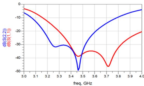
Figure 4. S11 & S22 versus frequency of the proposed amplifier
