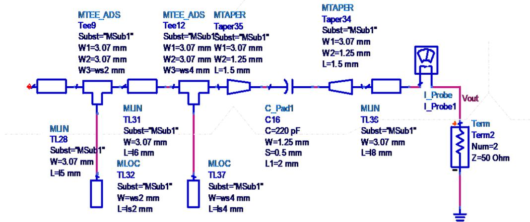
Figure 2(d). Output matching network circuit
