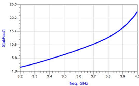
Figure 6. Stability Factor versus frequency characteristics
