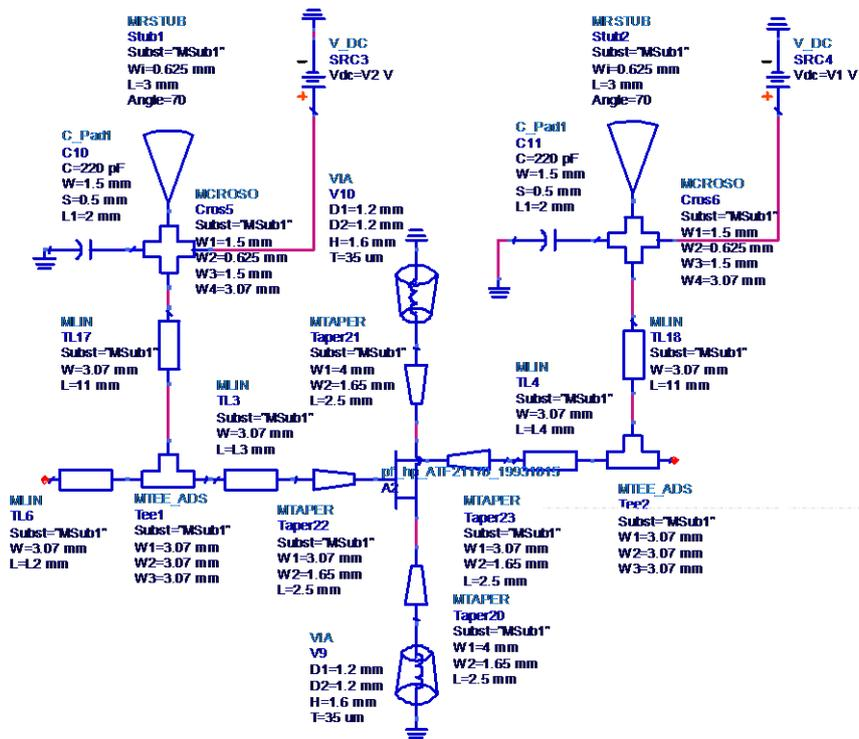
Figure 2(b). Biasing circuit
