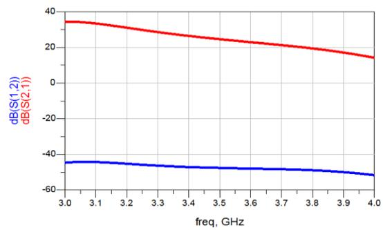
Figure 5. S12 & S21 versus frequency of the proposed amplifier
