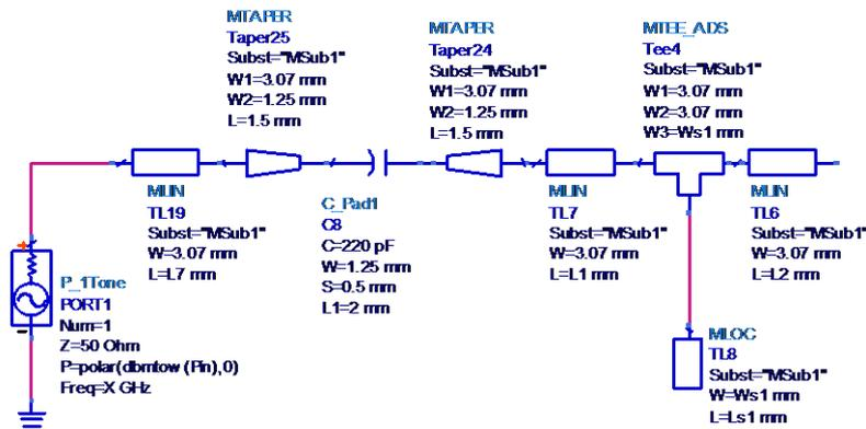
Figure 2(a). Input matching network circuit
