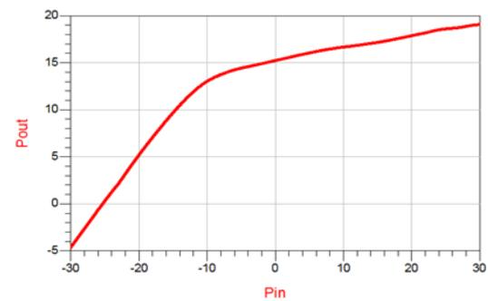
Figure 7. Input power versus output power for 3.5 GHz
